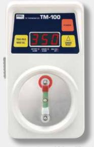
Wide temperature range \*0-700°C (1292°F), as is necessary for soldering work. The tolerance stays in the range of ±0.5% of the full scale (excluding sensor error). The sensor's structure makes for easy tip placing. It achieves stable & accurate measuring within seconds, regardless of shape, or angle of tip. Easily replaceable sensor.
